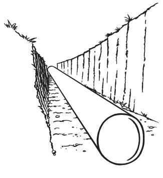
When ya' in the rural blocks take the **FFP** approach... but use your common sense... big boulders and organic material (lumps of turf) don't work as bedding, get 'em out. Use loose selected as dug material in the backfill zones, remove the big boulders as they could damage any plastic pipe!
