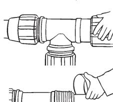
6. Open the split ring and mount on the pipe with larger side against the bushing. Ensure that the bushing and the split ring meet the body of the fitting.
