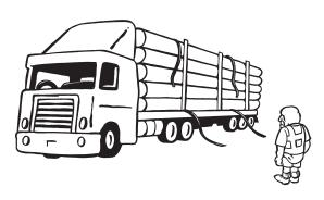
Check the pipe when you get 'em on site. Unload carefully. **Never** tip 'em off. When ya unstrap the load keep **way back** from it cos PE Pipe is as slippery **as an old eel!**
