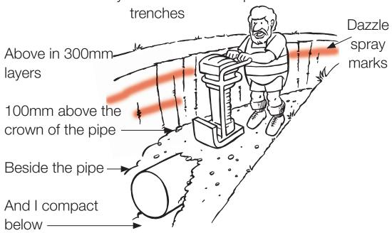
Compacted granular bedding/aggregate surrounds the pipe and up to a minimum 100mm above the pipe. Then I use selected ordinary backfill. I compact with my machine below, beside and above the pipe in layers of 300mm until I get to the top surface.
