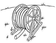
There can be a lot of stored energy in coiled PE pipe. Make sure the pipe-end is strapped down tight and the brake is on securely! Here's another way to do it... 125mm PE pipe made into coils then placed onto a pipe dispensing trailer.
