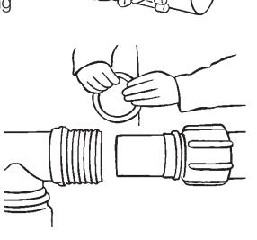
3. Insert the pipe into the body of the fitting until it meets the interior step of the fitting body. Then draw the seal ring and the bushing close to the body of the fitting.
