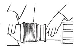
**4.** Tighten the nut with the wrench until the seal ring and the bushing enter the fitting and reach the rest position.
