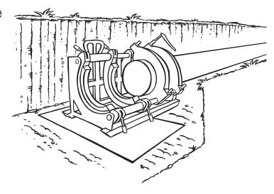
Place a thick large steel plate in the base of your level excavated pit that you are going to be working in...
