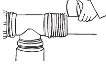
7. Screw the nut tightly towards the body of the fitting. For final tightening use a Plasson wrench with a maximum handle length of 40-46cm. Although the nut should be closed tightly, there is no need for it to travel the full thread length.
