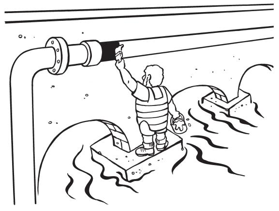
Hey, black pipes are the best to use outdoors cos black reflects the ultra voilet rays better. U.V. attacks coloured PE pipe real quick! If you need to use striped or colour skin pipe for some reason, paint 'em with a light coloured acrylic paint... The light colour paint will reflect the heat in those hot summer months.
