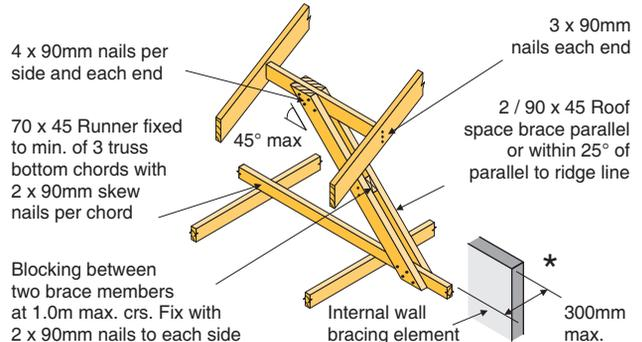
\* Not required when a ceiling diaphragm complying with Clause 13.5 of NZS 3604:2011 is used.
