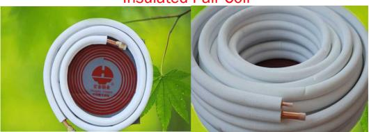
Application: The insulation is a double layered cross linked polyethylene closed cell foam. The insulation tube is extruded to ensure close tube contact to enhance dew point proofing properties. The insulation is covered with embossed polyethylene film to prevent the foam creasing. The insulation tube is good for Anti-UV, heat resistance, low water absorption. Insulated copper tube is mainly used for Installation of Air Conditioner, available in standard with lengths of 3-30m.
