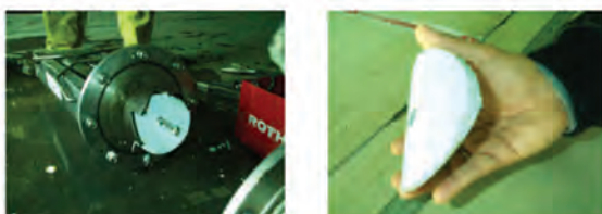
Figure 7.16: Use of a hole-saw cutter in the tapping machine results in a cleanly cut coupon
