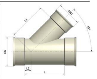
Note: \* DN100 & DN150 branches are available for PVC & VC connections.
