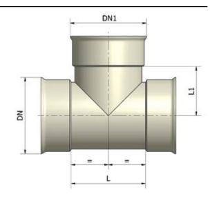
Note: \* DN100 & DN150 branches are available for PVC & VC connections.
