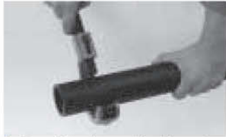
1 Roughly clean pipe(s), cut at right angles and trim edges
