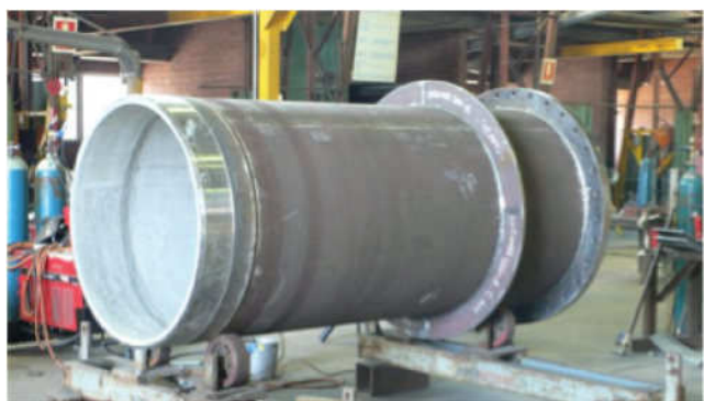
Figure 3.4 – DN1200 steel flange spigot connector with thrust flange, prior to coating and lining in the workshop
