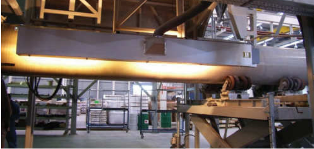
Figure 1.3 – FLOWTITE™ pipes being cured with infra red heat
