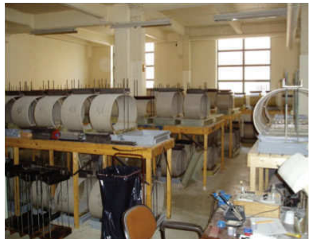
Figure 3.6 – Strain corrosion testing of FLOWTITE™ GRP pipe samples
