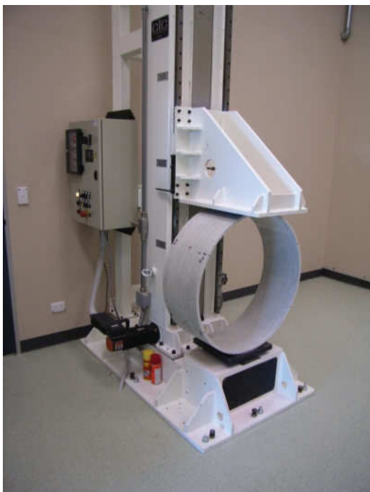
Figure 3.5 – Pipe stiffness test
