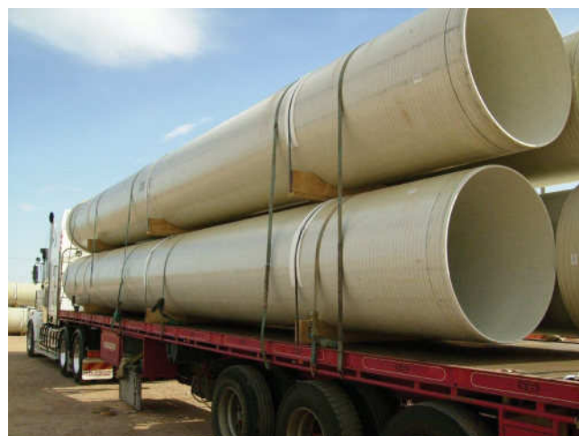
Figure 7.1 – Semi-trailer with FLOWTITE™ pipe packed with shaped timber bearers, ready for transport to site
