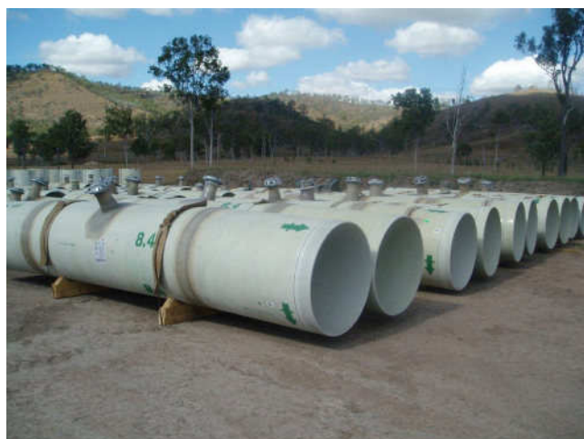
Figure 4.2 – Flanged off-takes for air valves and scours (Note stub flanges and backing plates, which are the preferred option)
