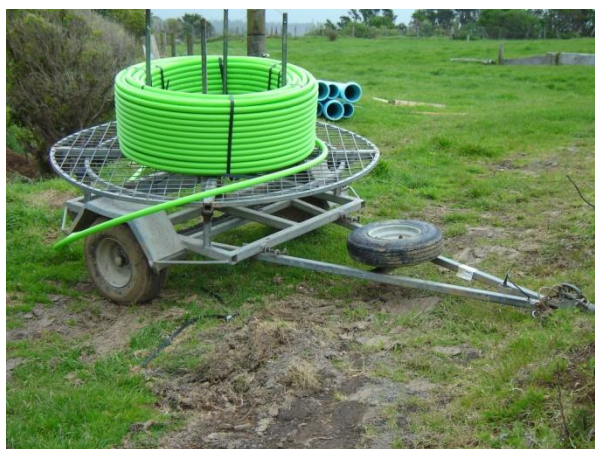
DN 32 PE telecommunication duct in a 500m coil on a coil dispensing trailer
