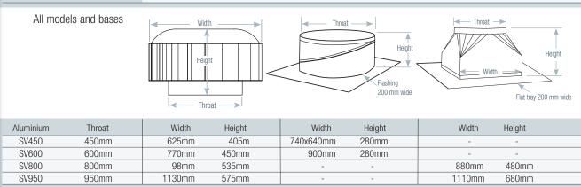
Bases Ampelair ventilators models: SV450 and SV600 are supplied complete with a Variable Pitch – Aluminium base to suit any application. Ampelair ventilator models: SV800, SV950 are head only units but can be supplied with Heavy duty Square to Round bases made from Zincalume.
