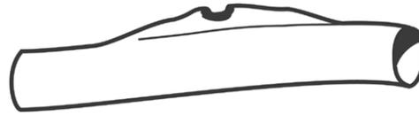
This is a typical ductile failure mode caused by the internal pressure exceeding the pipe's capability, a number of factors can cause it, including:
