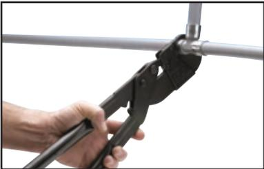
3. Clamp approximately 2mm in from the end of the fitting, close the tool handles completely to the stops provided, and hold firmly for around 2 seconds then release.
