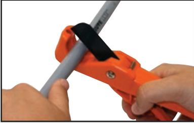
1. Cut the pipe with the Buteline pipe cutter.
