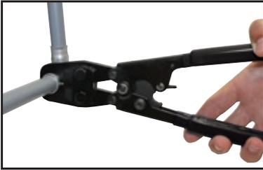
3. Clamp once only, approximately 2mm in from the end of the clamp ring. Close the clamp tool handles completely, holding firmly until the ratchet allows the handles to open and release.
