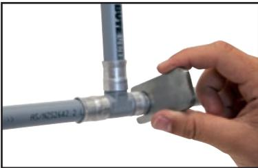
4. Use the gauge provided to check that the full clamp force has been achieved. If the gauge does not pass over the ring, the ring is under-clamped. It is important that the gauge passes over the clamp ring.
