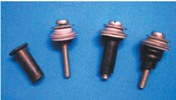
When fibreglass sheeting is lapped onto metal sheeting a T17 coarse threaded self drilling screw with a 32mm Weatherlok Seal fastened into the top of the rib, provides a firm seal in the lapping joint. The table below indicates the recommended spacing for side stitching fasteners.
